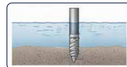
Piles driven into waterbed for stability
