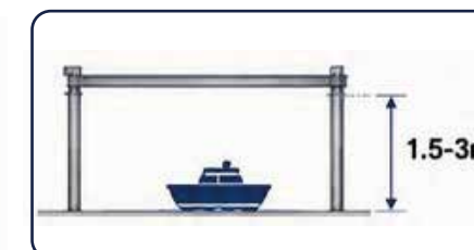
Elevated clearance 1.5-3m for boat passage & fishing
